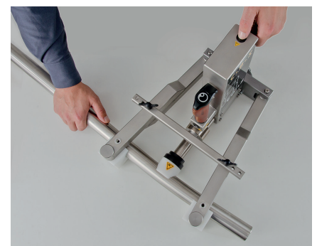
Bending of a 42 mm pipe
